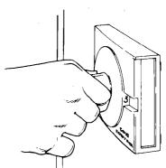
Plug cord into wall outlet and return cold control to original setting. Check to see that the signal light glows. Return food to the freezer.
